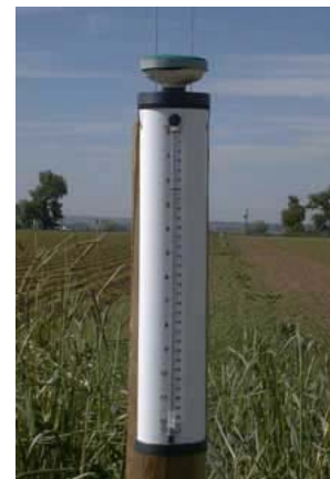
Atmometer placed between irrigated fields.
